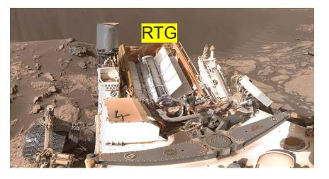
RTG is the only steady power supply for space probes running for over 30 years.
