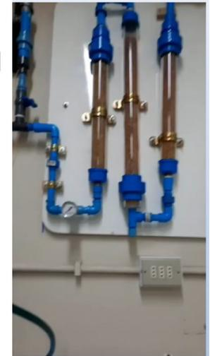
Redesign and assembly of the adsorption equipment
